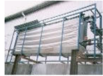
Liquid by-product recovery and re-use using membranes
